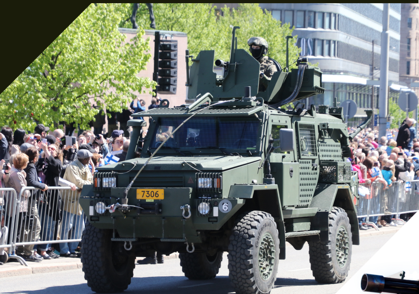
Finnish RG32M armed with M134 Minigun mounted on Platt MR550 protected Ring Mount
