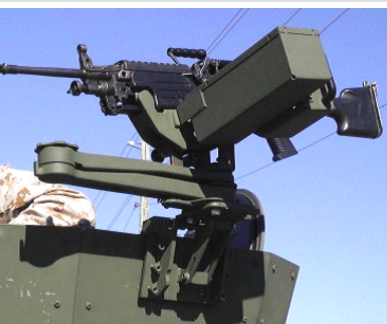
Clamp-on 30 bolted on the vertical shield surface (left); 'B' Pillar Clamp-on bolted on the roll bar (right)
