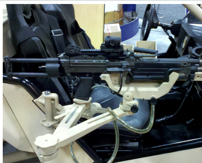
Clamp-on 30 bolted on the vertical shield surface (left); 'B' Pillar Clamp-on bolted on the roll bar (right)
