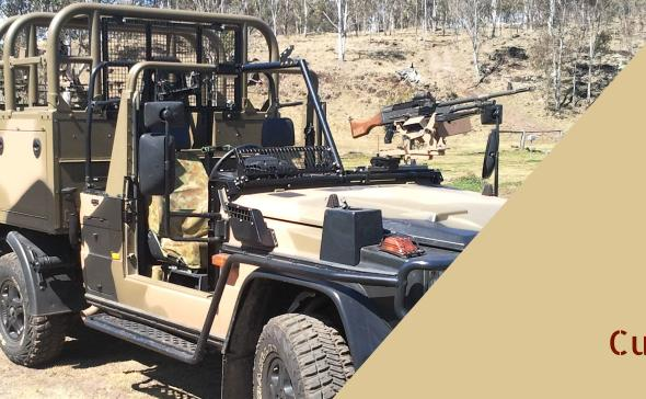
The Platt Rail Mount is an innovative, highly versatile and flexible front weapon mount especially suited to the front passenger position in soft-skinned, open-topped vehicles for patrol, reconnaissance and special operations. The lightweight Rail Mount is instantly adjustable for left or right-handed gunners and multiple arcs of fire.
